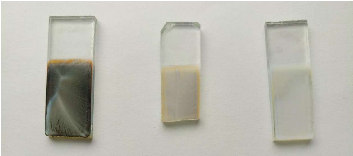
Figure 4: Photodeposited Cu/TiO 2 samples from acetate precursor in ethanol solution. Deposition times from left to right: 45, 20, 5 min
