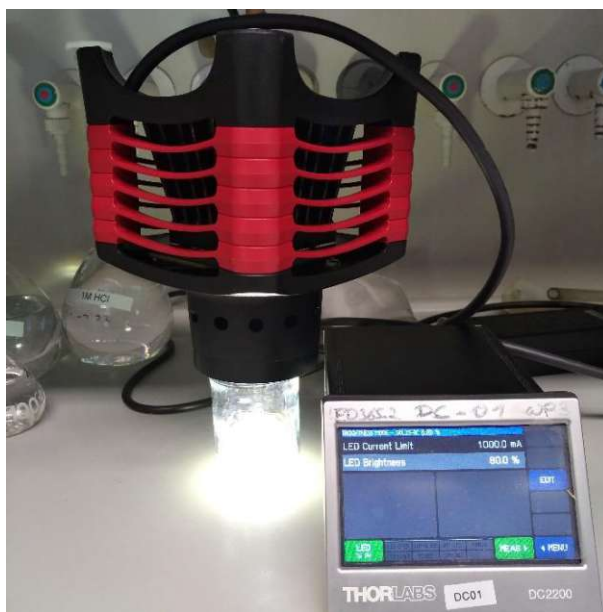
Figure 1: Setup for photodeposition of Cu onto BiVO 4
