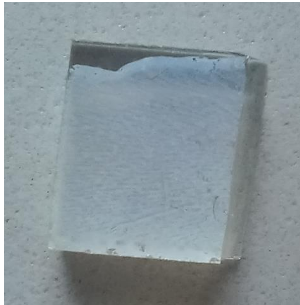
Figure 3: Photodeposited Cu/TiO 2 sample from aqueous precursor
