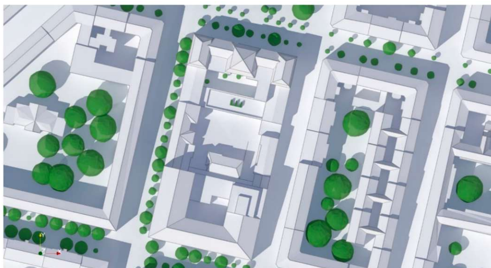
Figure 20. Shadow cast at Schuhmeierplatz School on the model day at 3:00 p.m. CEST, with the position of the greenery systems highlighted.
