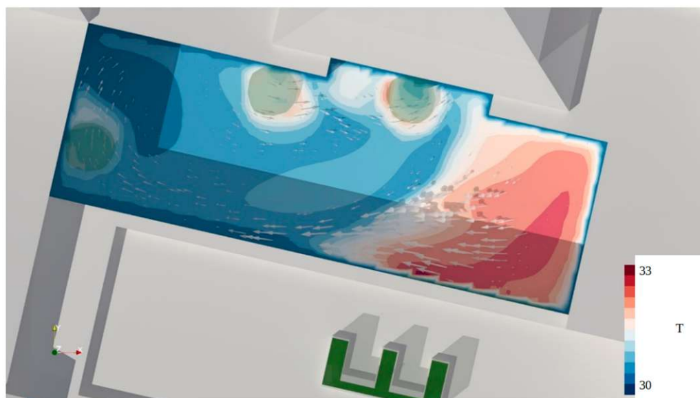
Figure 22. Air temperature ( ^{\circ}\text{C} ) at the level of the Schuhmeierplatz School living wall on the model day at 3:00 p.m. CEST.
