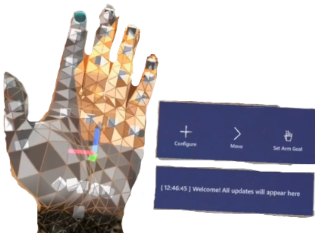
Figure 4: Overview of the supported modes - Configure (left), Move (middle) and Set Arm Goal (right).
