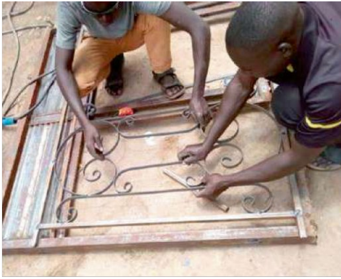
fig.16 Welding windows and grilles.
