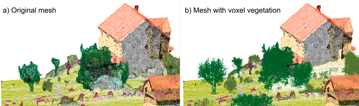
Fig. A.11. Comparison of (a) the original Hessigheim 3D mesh and (b) the modified Hessigheim 3D mesh with voxelized vegetation. Colored by classification. (For interpretation of the references to color in this figure legend, the reader is referred to the web version of this article.)
