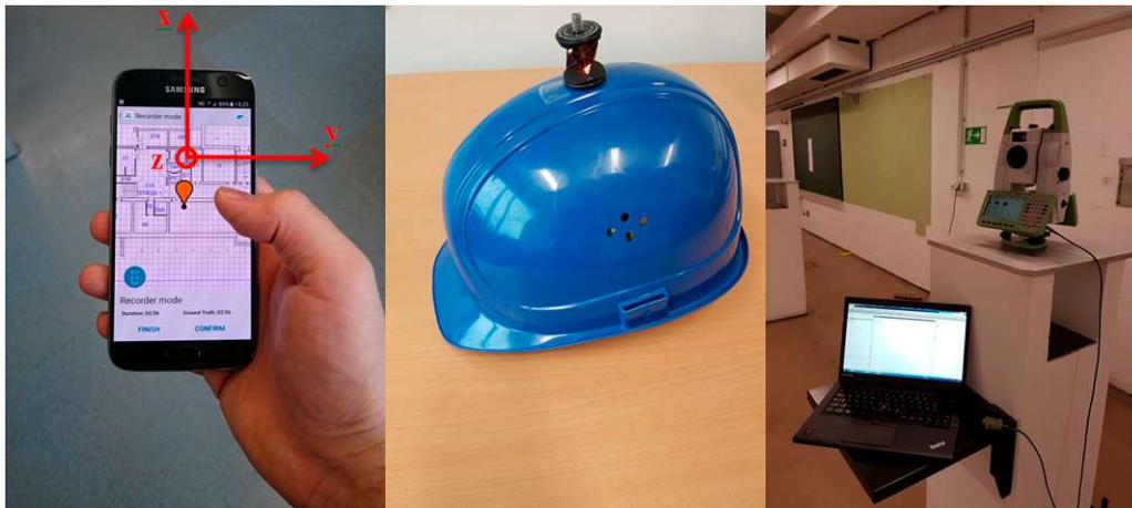
Figure 2. Used sensors and measurement setup: Samsung Galaxy S7 (Samsung, Seoul, Korea), smartphone running indoo.rs Mobile Toolkit™ to collect sensor observations (left). Helmet with 360°-mini-prism (middle) and Leica TS16 tracking the user (right).
