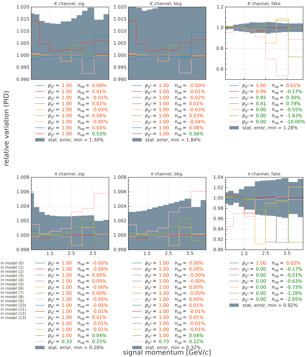
Figure 4.29: Relative shape variations of the templates due to hID uncertainties. Each template is affected by independent histosys modifiers, shown in different colours. These shape variations model together the desired correlation between the template bins. The hID selection is using the Reweighted variable with a working point of 0.9. The BDT output working point is set to 0.5.
