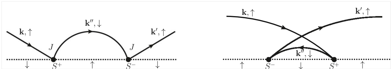
Figure 3.1: Lowest order Feynman diagrams for the Hamiltonian in Eq. (3.2), that contribute to the logarithmic resistivity contribution. The solid line (with conserved spin) denotes the conduction electron propagator. The dashed line denotes the impurity spin. The Feynman diagrams are inspired by Ref. [264].
