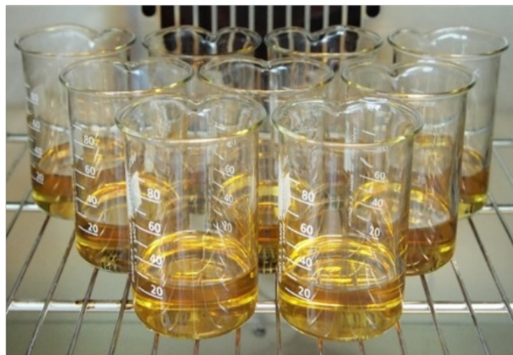
Figure 1.1: Alteration example: Open-beaker setup. Source: AC 2 T research GmbH.
