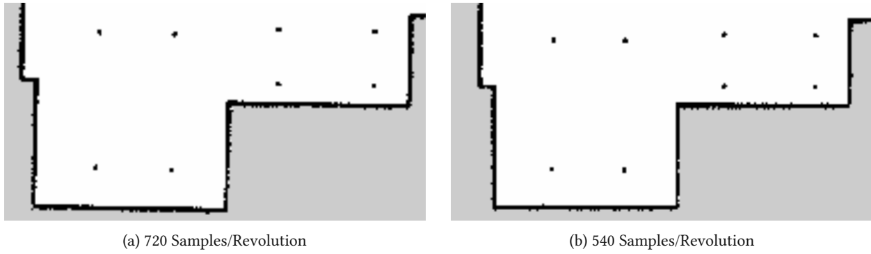
Figure 6.6: Maps generated with Gmapping-SLAM with different Samples/Revolution
