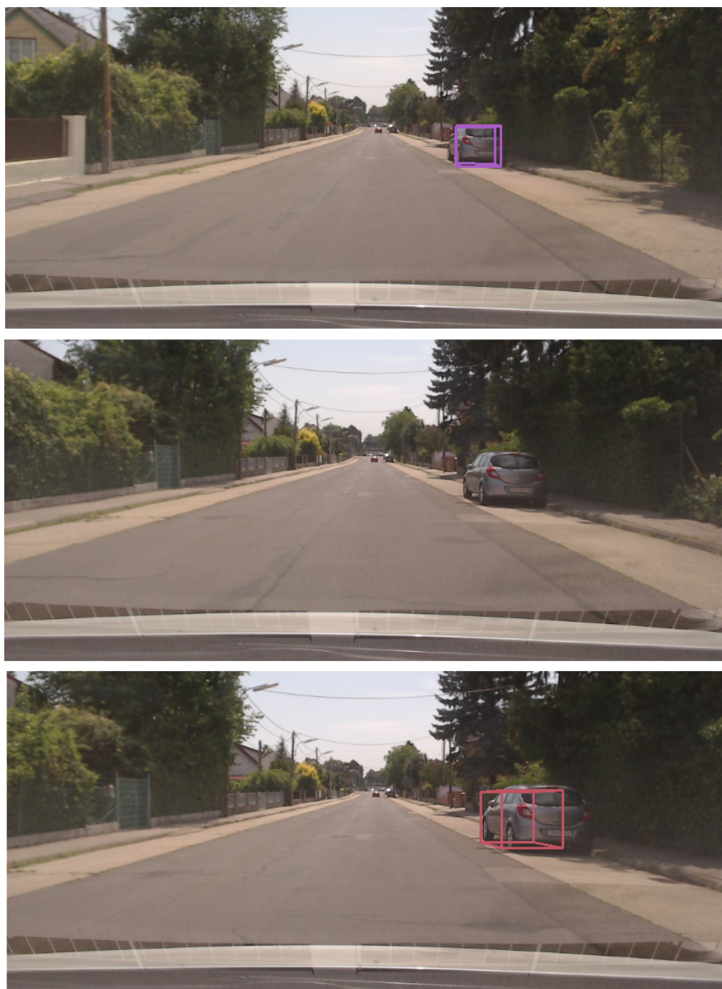
Figure 4.7: Qualitative results on the Bike2CAV dataset where a car is detected in the first frame, missed in the second frame and then detected correctly again but falsely identified in the third frame.
