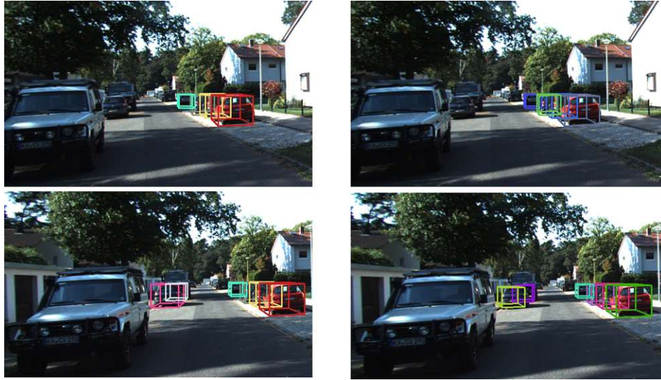
Figure 4.3: Comparison between proposed reID approach (left) and simple Kalman Filter (right) on the KITTI validation set.
