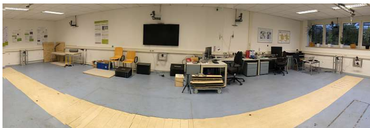
(a) Picture of the gait laboratory of Otto Bock. The walkway with the force plates aligned at the centre and infrared cameras can be seen as well as the marker on the floor before the force plates that indicate the light barrier that start the recording.
