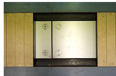
(b) The force plate underneath the beams can be seen in this picture. The beams are adjusted to fit each subjects walk and to ensure that only the heel strike of one foot is recorded by the force plate.
