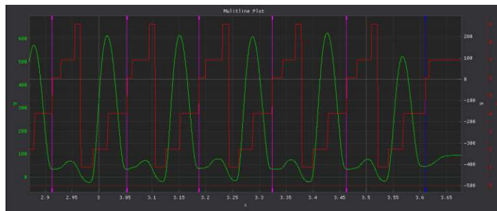
Fig. 4.6: Multiple steps in a recording. Initial contact is indicated by the vertical marker. Pink indicates that the step starting at given point in time might be included. Blue indicates that the step series has ended. The green signal is showing knee angle and the red one shows the rules that are currently active. Initial contact happens in that recording when the rule changes from four to six.
