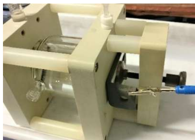
Figure 25 Side view of FlowCell including flat sample
