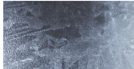
Figure 12 Visual appearance or top view of Sebisty steel zinc coated surface after surface photography (22)
