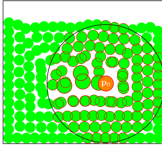
Figure 4.8: The effect of setting the kernel width to the boundary distance: particles near the center of the fluid body might have almost all particles as their neighbors. The kernel centered at \mathbf{p}_0 reaches all the way to the boundary, and all neighbor particles within the kernel are highlighted with red circles. The high number of neighbors increases the computational effort.
