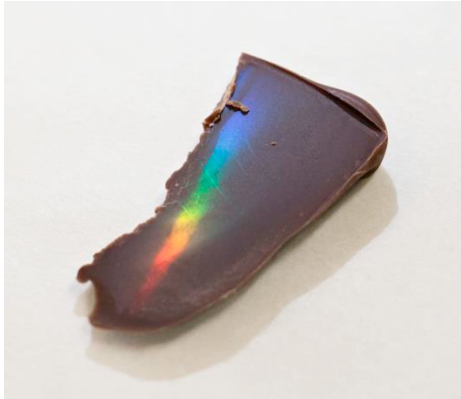
Figure 1. Chocolate exhibiting iridescence in rainbow hues due to the transfer of microstructures from a compact disc (CD) onto its surface. This phenomenon is a direct consequence of the interaction between light and the micrometer scale features on the chocolate, showcasing an experiment bridging science and the arts.
