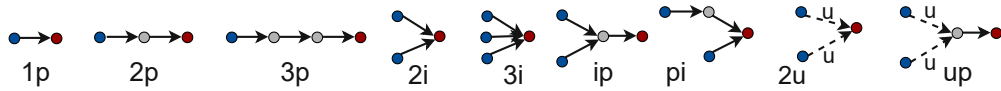
Figure 6.5: Query shapes considered in our experiments, where blue nodes correspond to anchor entities and red ones to answer variables; p stands for projection, i for intersection and u for union. The first five shapes are used in training.
