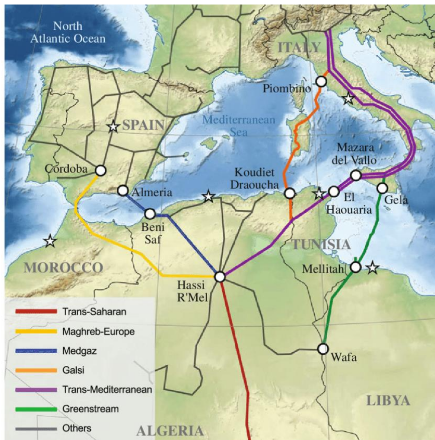
Figure 17. The existing gas pipeline network between Europe and North Africa can be used for H 2 transport. Source: Research Gate, n.d.
