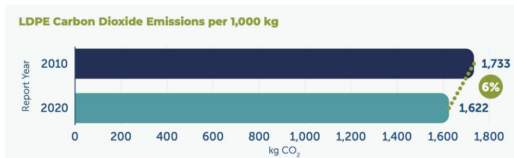
Figure 18. LDPE carbon dioxide emissions per 1 kilogram ( ACC, 2022 )
