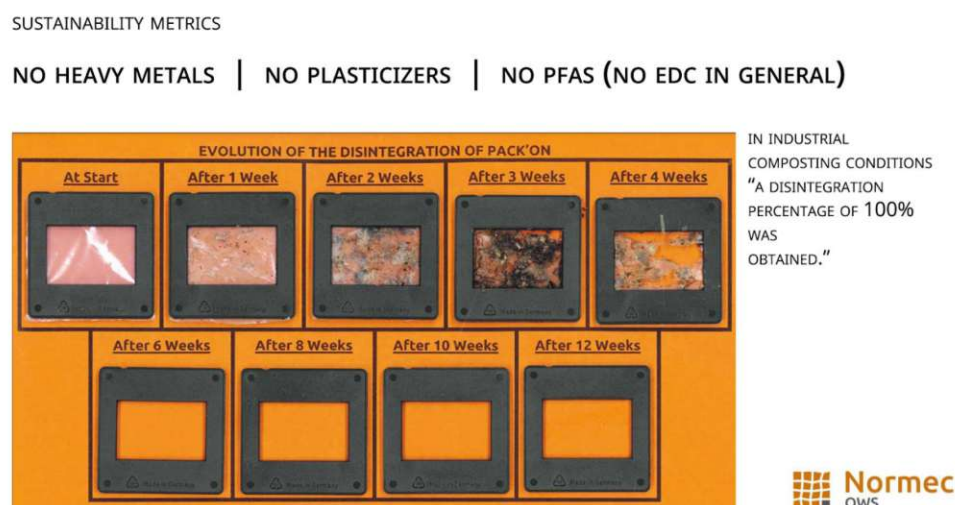
Figure 15. Evolution of the disintegration of Pack'On performed by Normec (Lam'On Presentation, 2024)
