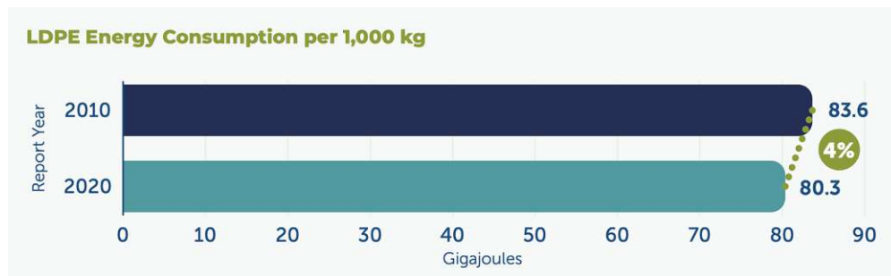
Figure 19. LDPE energy consumption per 1 kilogram ( ACC, 2022 )
