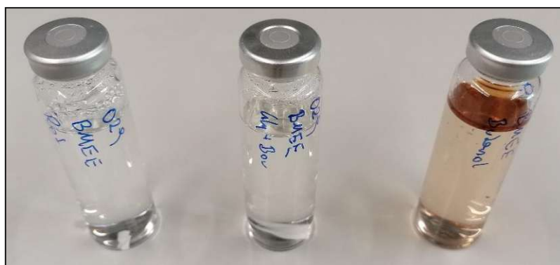
Figure 57: Degraded TPTU-BMEE samples with excess of 1-butanol (right), glycerol and BDB (middle) and without any additions after storing in PBS buffer solution (4x) at 90 °C for 7 days.
