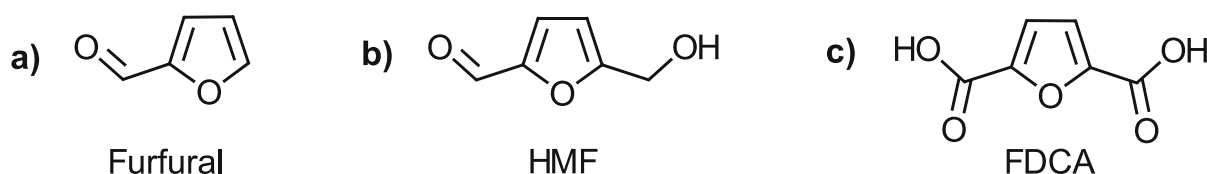
Figure 16: Chemical structures of renewable furan-based precursors and monomers: Furfural (a), 5-(hydroxymethyl)furfural (HMF, b) and furan-2,5-dicarboxylic acid (FDCA, c).
