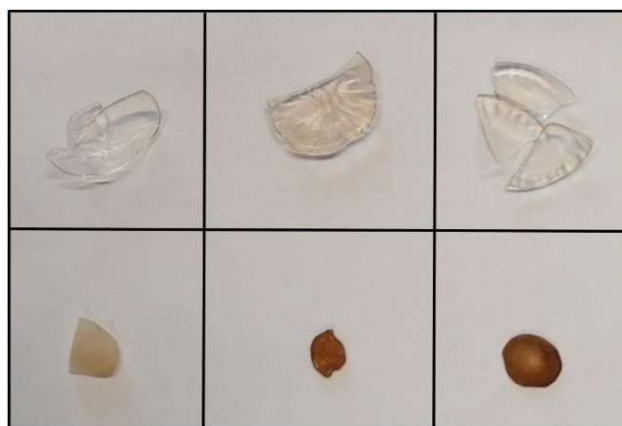
Figure 54: Non-soluble TPTU-BDB after degradation of 14d (left) and 21d (middle) in PBS and after 7d (right) at pH=10. Top row shows insoluble but swollen samples in hexafluoro-2-propanol. Bottom row shows degraded samples after drying.
