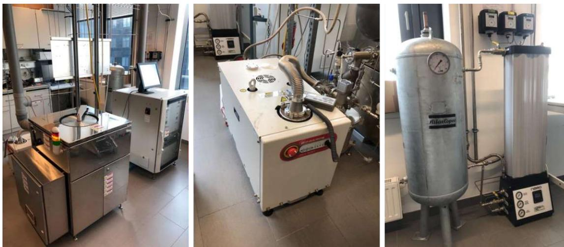
**Figure 2.1:** ALD-setup at TU Wien (E165, IMC) – from left to right: Picosun R200 Advanced ALD reactor with human interface; Edwards iXH 100 dry pump; ECO GEN 2 nitrogen generator
