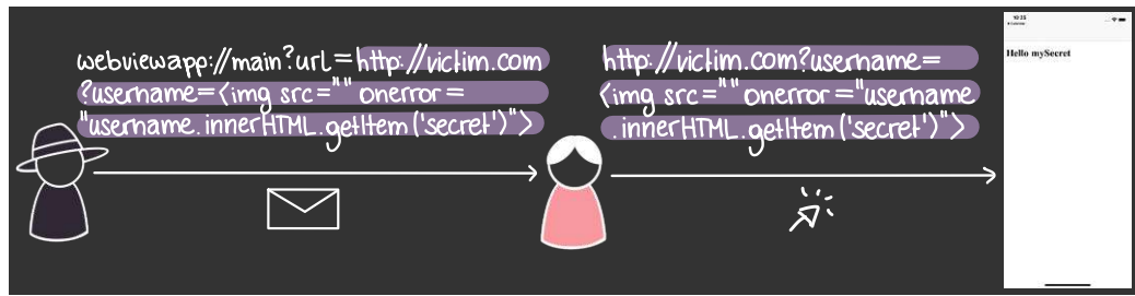
Figure 4.10: Procedure of a CSRF and XSS within a WKWebView.
