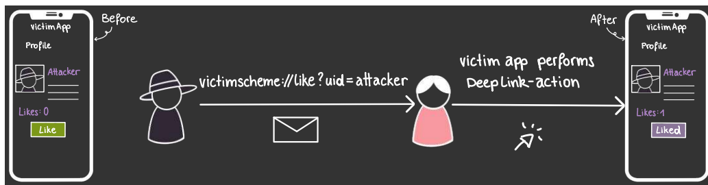
Figure 3.4: Schematic representation of Malicious API Usage. The attacker sends a malicious deep link to the victim, such that the victim app executes the like action on the profile of the attacker without the users interaction.
