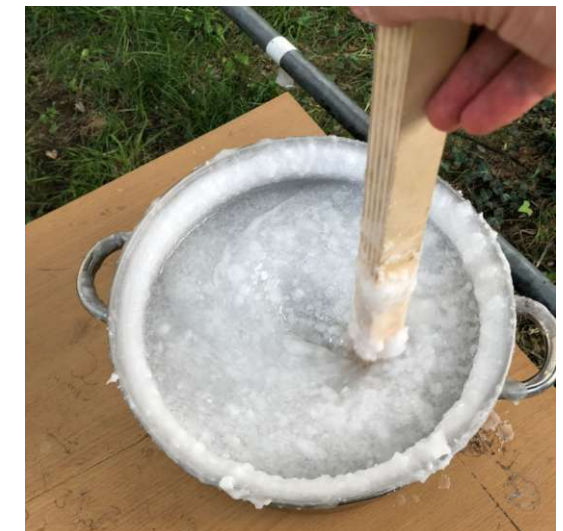
Fig.311. While casting the wax is continuously stirred
