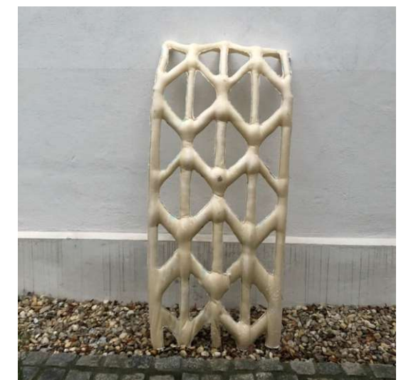
Fig.313. When solid, unnecessary textile can be removed
