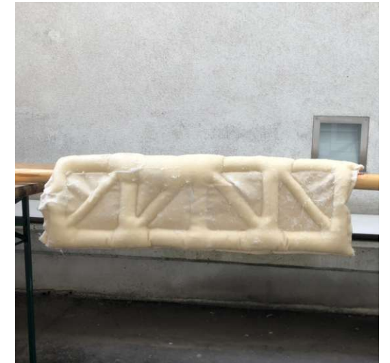
Fig. 159. The object had to be hung to solidify to preserve the geometry
