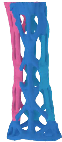
Fig.321. The exemplary filling process of one structure, dark blue first cast; light blue second cast; pink last cast
