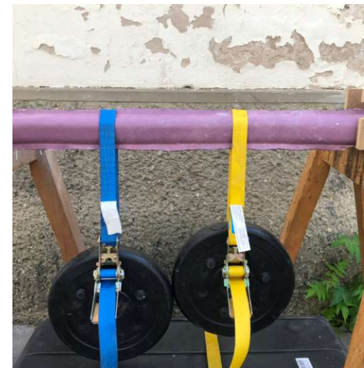
Fig.153. In the new stress test setup the load was applied at 1/3 & 2/3 of the length
