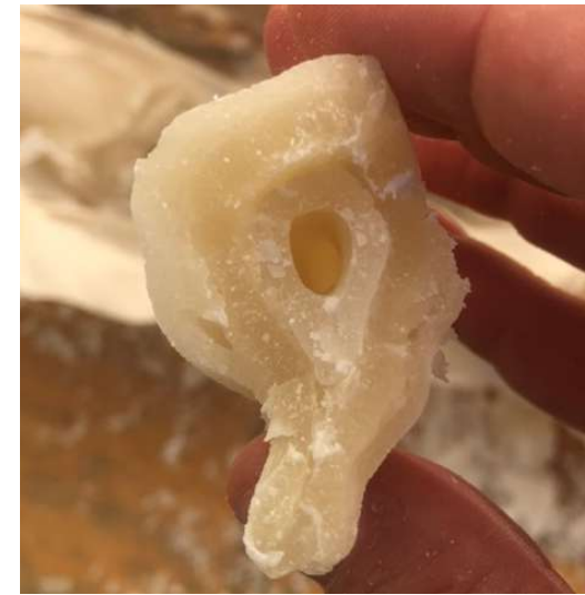
Fig.323. The casted wax had multiple layers which were only loosely connected
