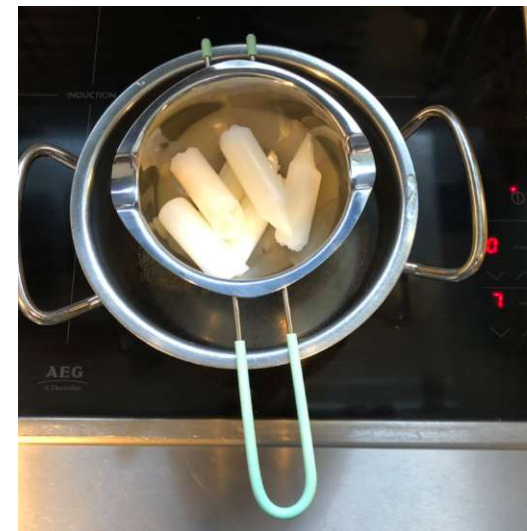
Fig.60. The wax was heated in a water bath
