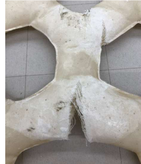
Fig.139. The object failed when the textile tore
