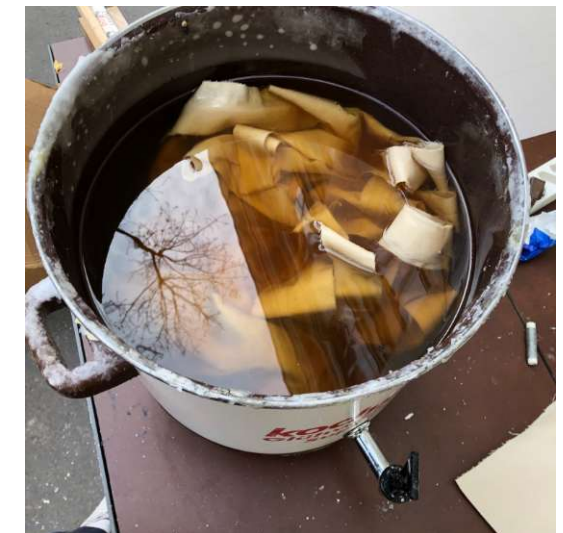
Fig.292. The textile was soaked with wax
