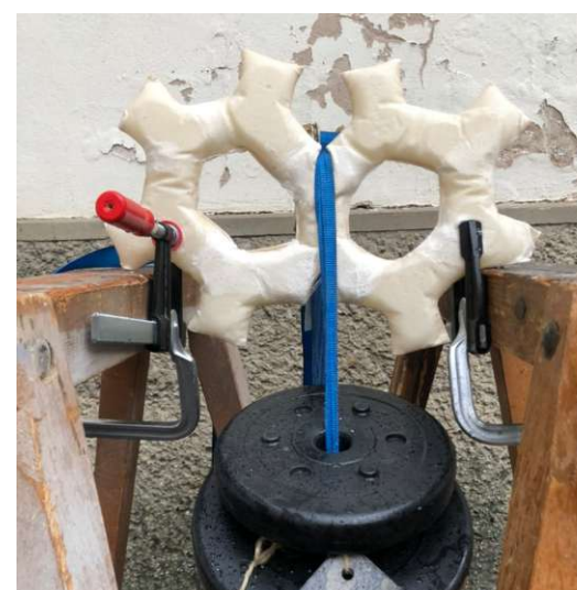
Fig.137. The object failed at 51,2kg
