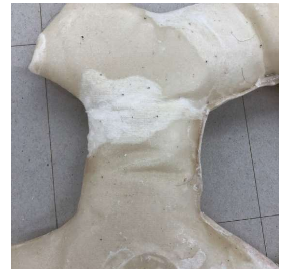
Fig.142. The object developed white spots in heavily stressed areas
