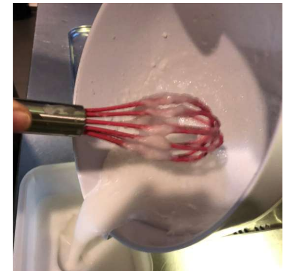
Fig.72. Foamed wax is poured into the formwork
