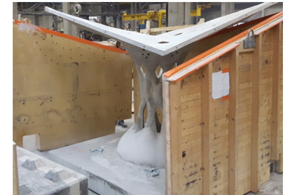
Fig.40. The wooden substructure for the casting process
