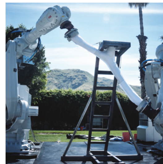
Fig.43. Robots were used to cast the modules
