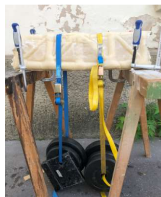
Fig. 320 Models were loaded at 1/3 and 2/3 of their length
