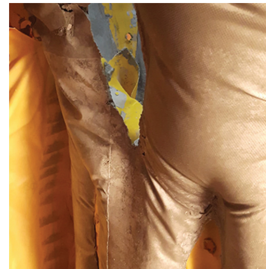
Fig.41. Wrinkles in the casted shape
