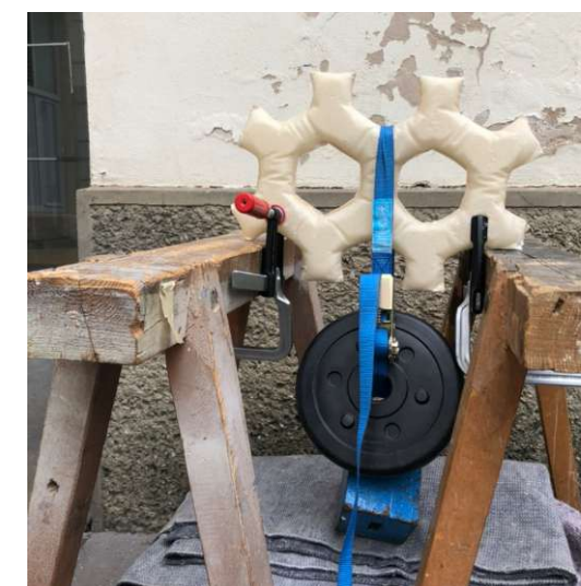
Fig.136. The first deformation at 38,8kg
