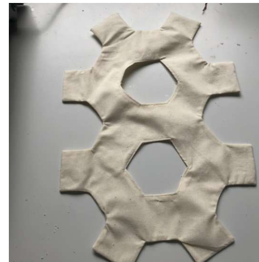
Fig. 127. The finished formwork
