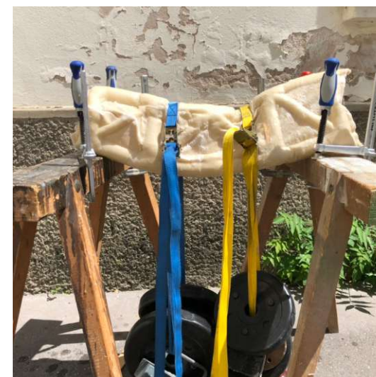
Fig. 162. The object failed and deformed at 51,8kg
