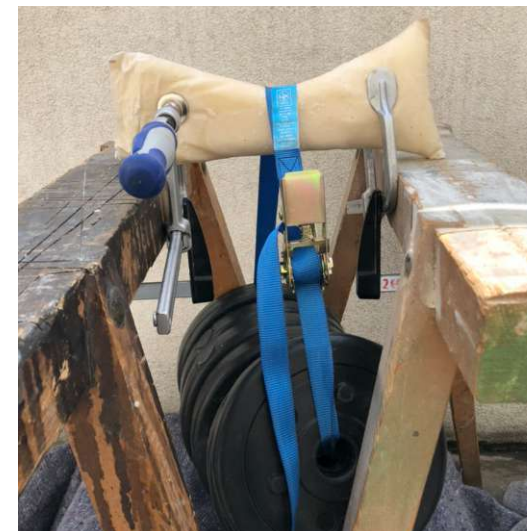
Fig. 122. The first deformation at 20kg
