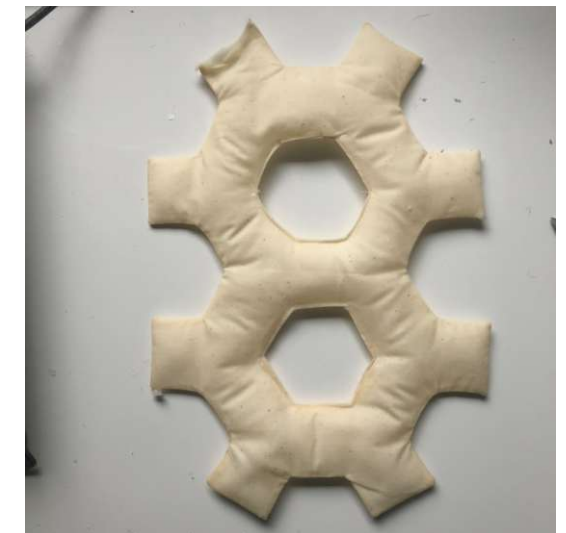
Fig. 128. The formwork was soaked in wax and inflated with air
