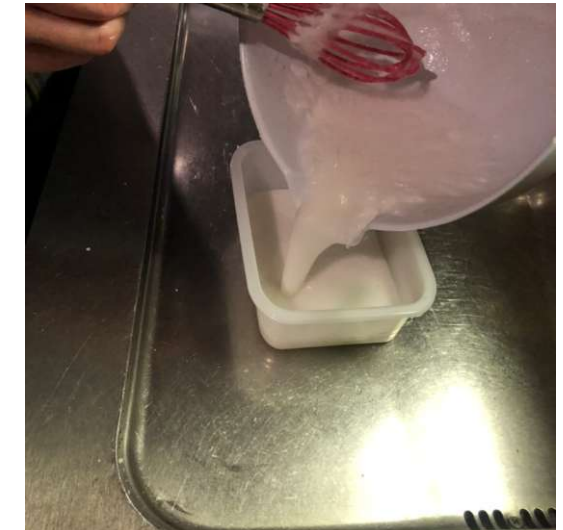
Fig.78. Foamed wax is poured into the formwork
