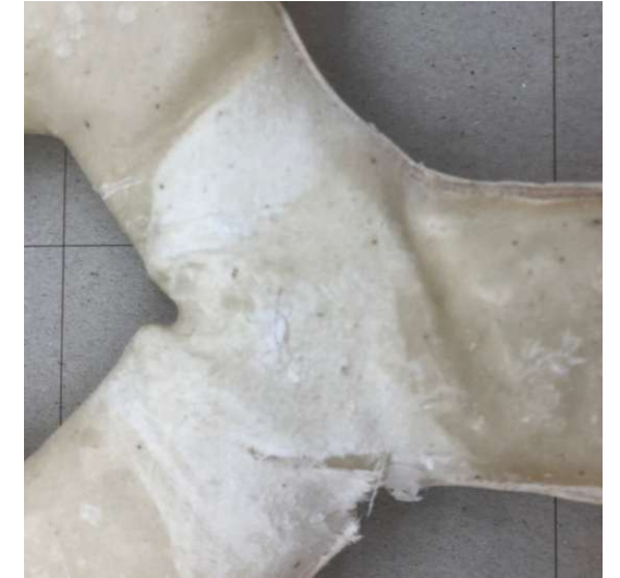
Fig.140. The upper tear in the textile
