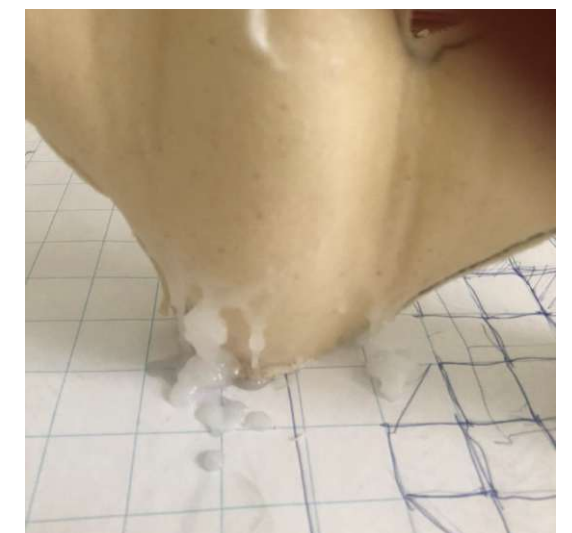
Fig.205. A detail of the lost wax due to heating
