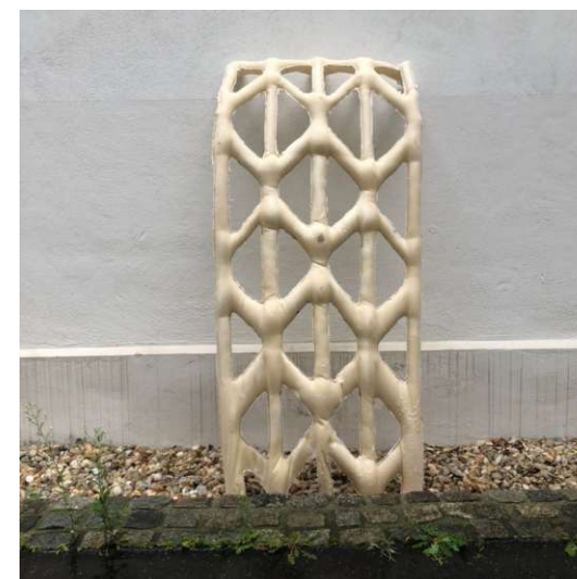
Fig.198. The structure erected and removed from redundant textile
