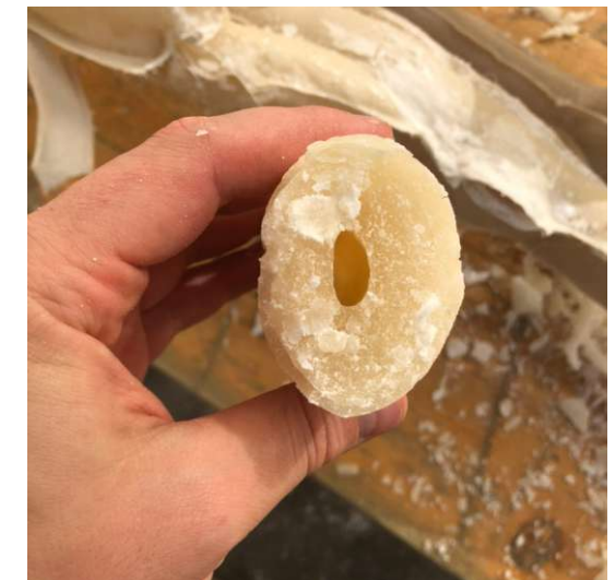
Fig.282. An enclosed air bubble in the middle of the beam
