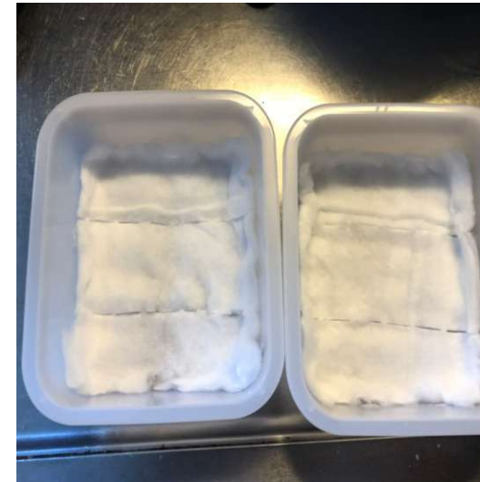
Fig.89. Cotton is place into the formwork and soaked with wax
