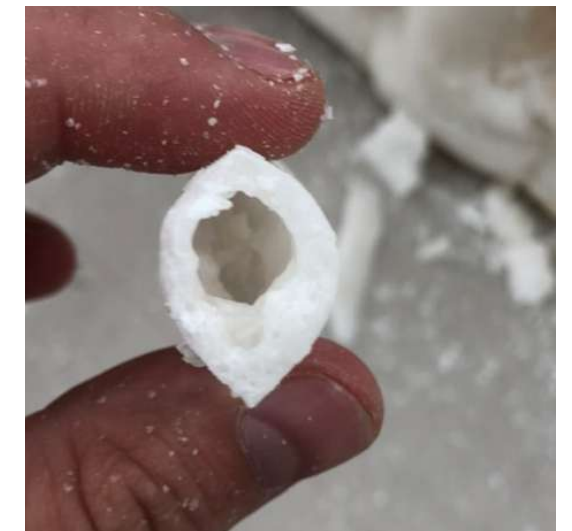
Fig.167. A common casting mistake
