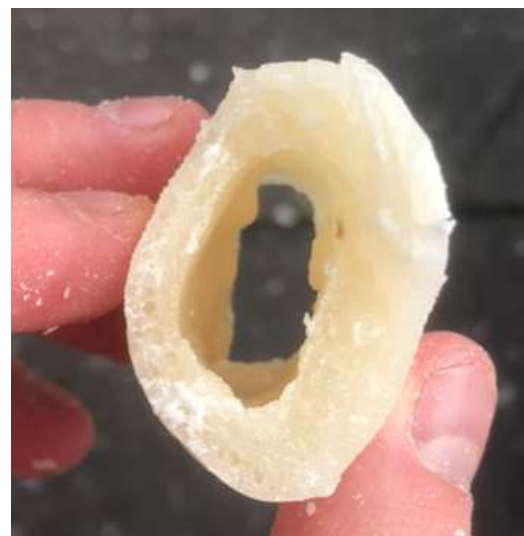
Fig.327. A trapped air bubble in a beam
