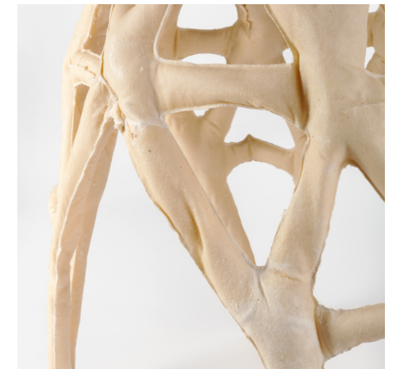
Fig.262. Horizontal beams were hardly connected to the structure
