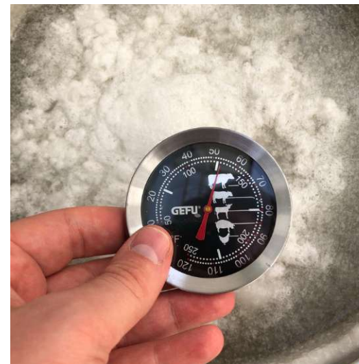
Fig.310. Wax is heated to a temperature slightly above the melting point
