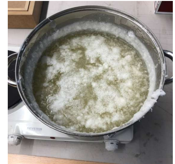
Fig.146. The wax was cooled down to have a higher viscosity
