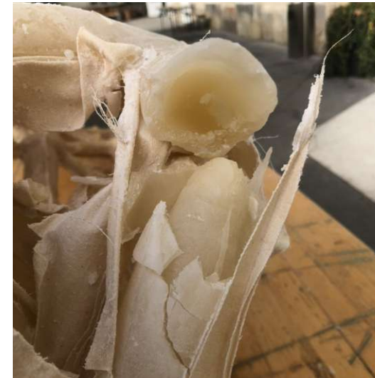
Fig.279. The casted wax did not form a uniform material
