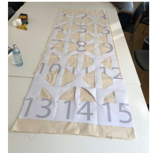
Fig.183. The pattern was cut out and transferred onto the textile
