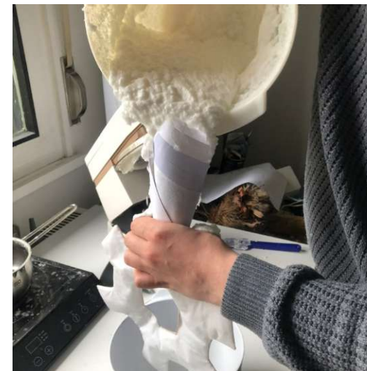
Fig. 129. The wax was poured into the formwork with a funnel
