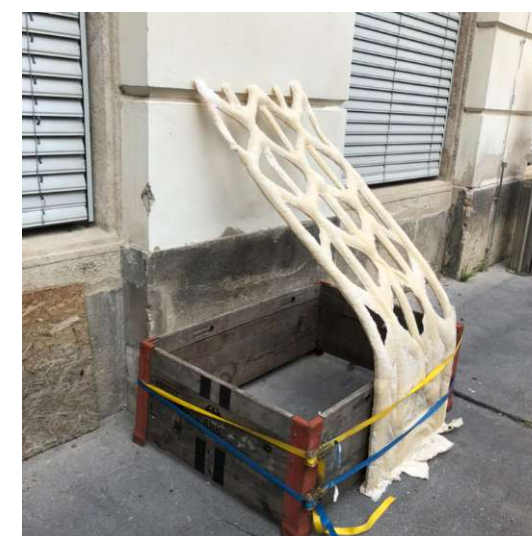
Fig. 193. The structure failed due to its 2D geometry
