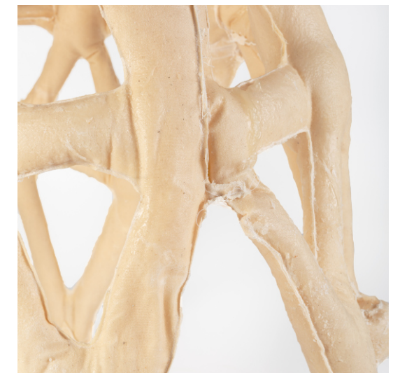
Fig.264. The joint on the side were insufficiently filled
