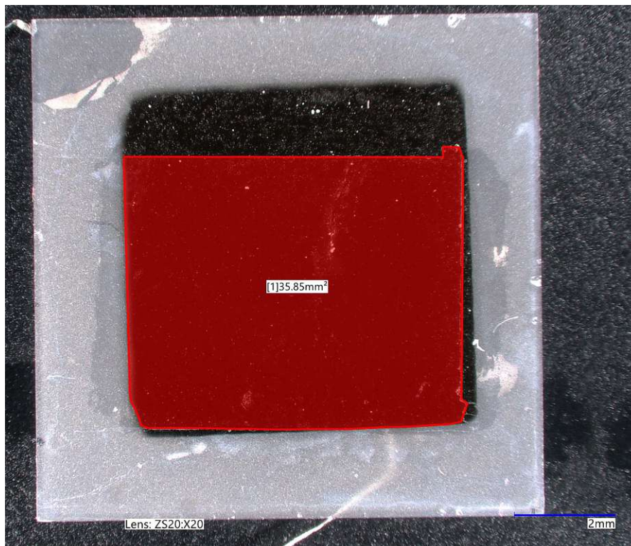
FIGURE 3.6: Microscopic image of a half-cell battery featuring a Ti/Pt thin layer coating atop an STO thin film (highlighted in red with area of 35.85 mm 2 ), placed on the YSZ single crystal
