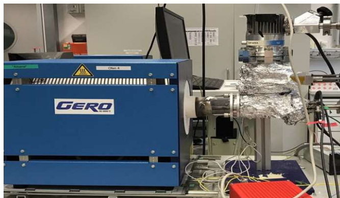
(a) The entire setup contains the furnace and outer tube covered with heating wire, that are shielded by an aluminum layer to prevent heat lost
