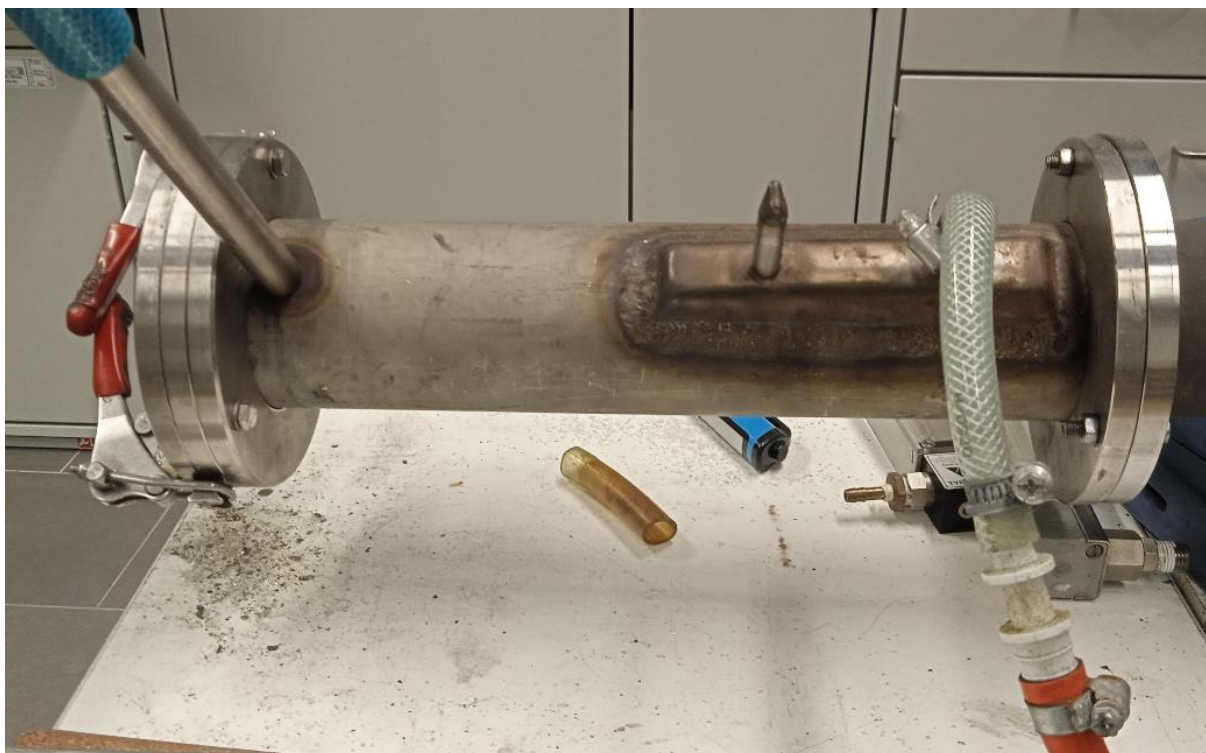
Figure 23: Gas quenching unit at the entering zone of the sintering furnace
