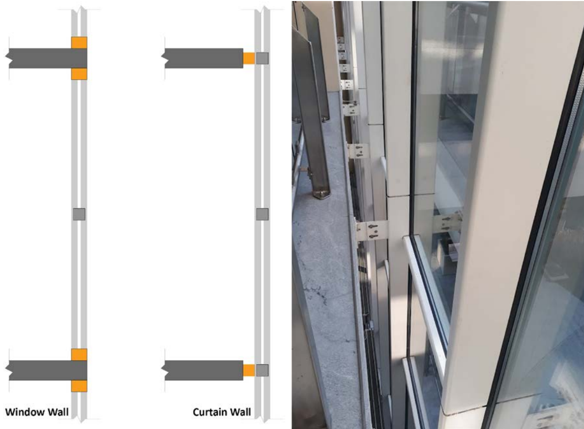
Figure 14. Left: a schematic drawing showing the difference in where the loads of a window wall vs a curtain wall apply to primary structure/slabs; right: an example of a curtain wall in the AKH building, Vienna. Source: the researcher
