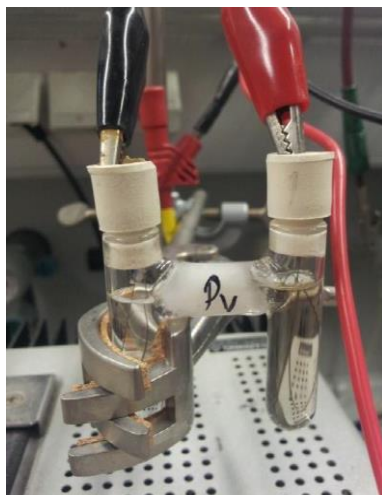
Figure 7: experimental setup for the single-crystal growth via electrocrystallization
