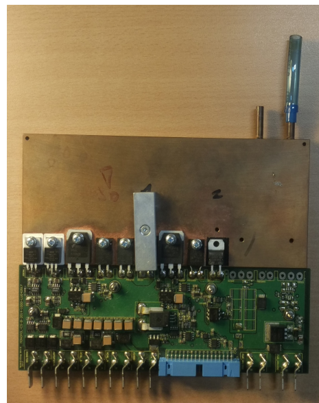
(b) A cooling element after assembly fitted with a power supply printed circuit board (PCB).
