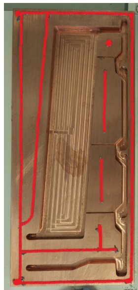
(a) Soldering pattern used (red).
