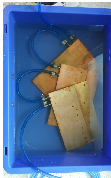
(a) Test setup for pressure tests conducted with a pressure of 4.5 bar in a water bath.
