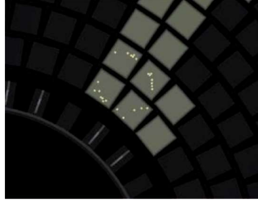
(b) Photon ring originating from a cosmic muon passing through ARICH.
