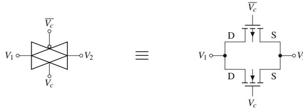
Figure 5.5: Internal structure of the Transmission gate. For  $V_c = GND$  both transistors prevent charge transport while for  $V_c = V_{DD}$  both fully conduct. The Transmission gate is thus the equivalent to a common switch, which propagates current in both directions.
