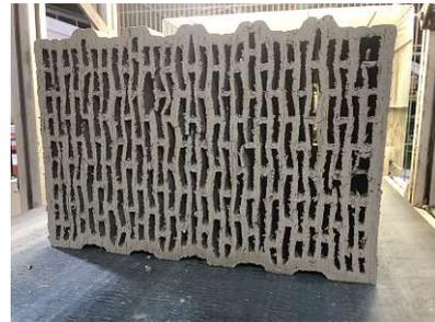
Figure 19: Picture of the cut brick.
