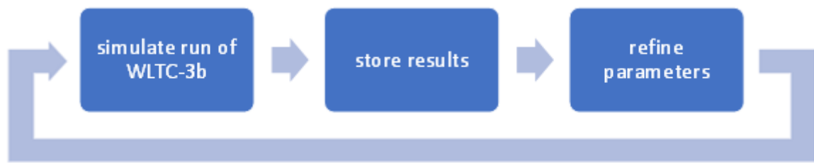
Figure 3.18: The work flow of a numerical optimisation process, heavily simplified.
