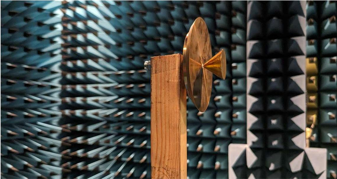
Figure 3.10: Measured UWB CMP antenna
