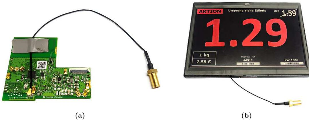
**Figure 5.4:** Connectorized ESL 4: (a) PCB and (b) assembled device
