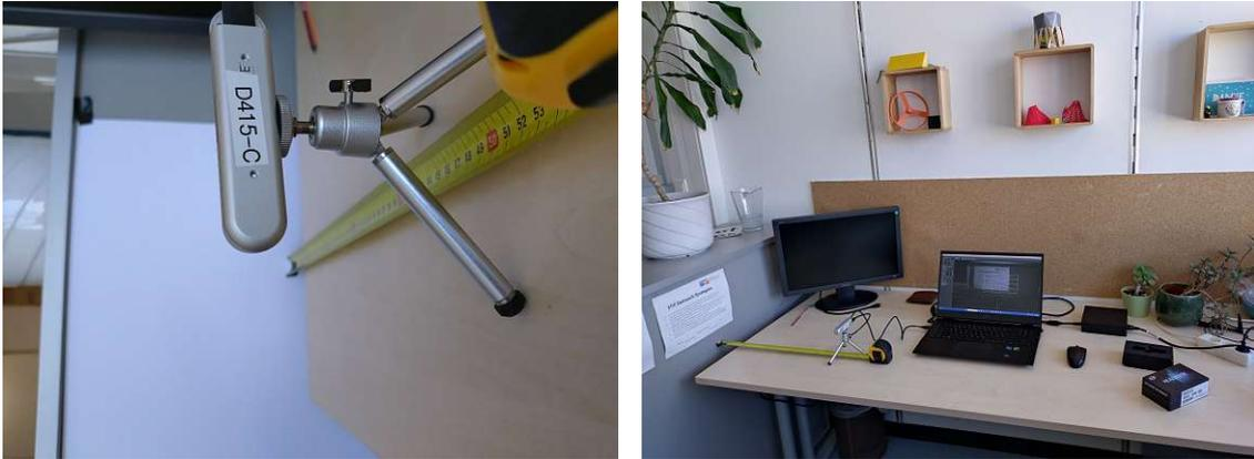
(a) Calibration distance measured by tape
