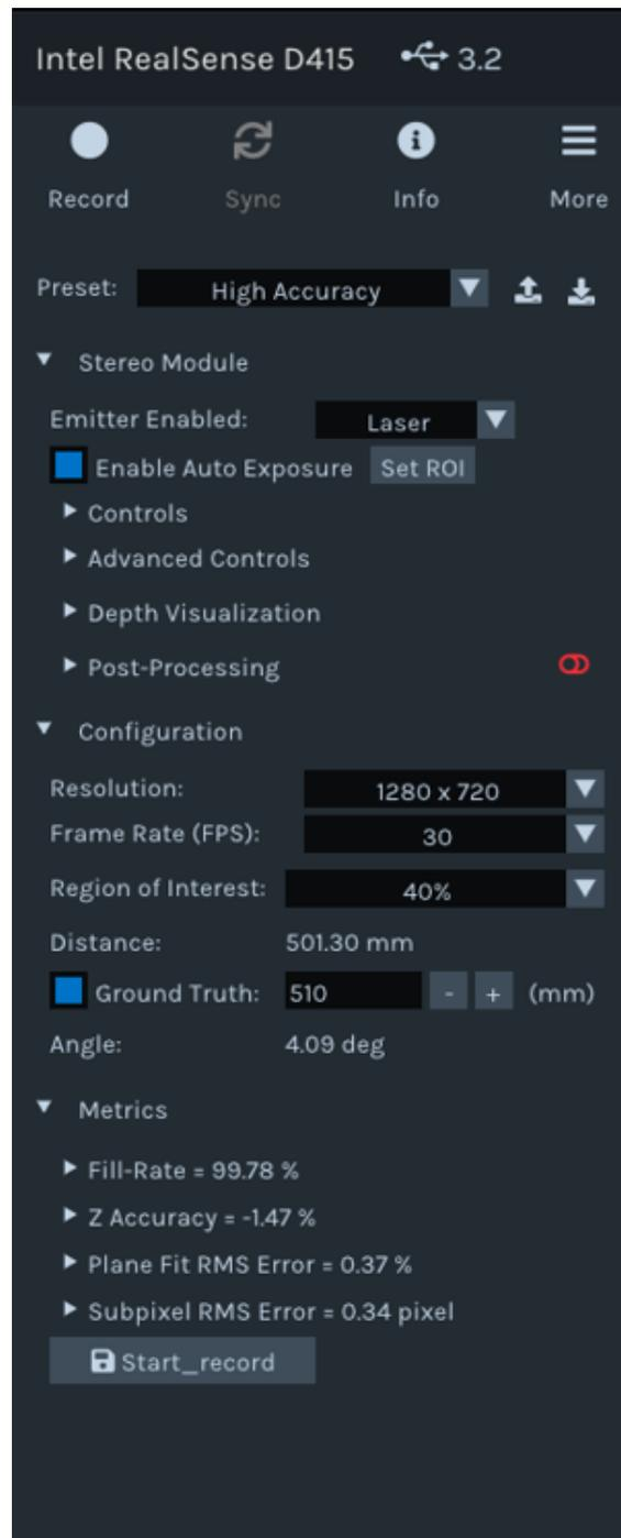
Figure 4.4: RealSense Viewer High Accuracy Preset
