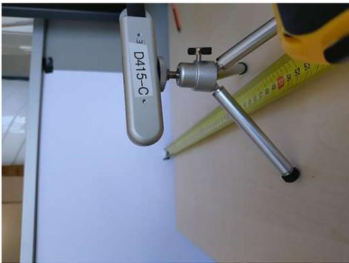
(a) Calibration distance measured by tape
