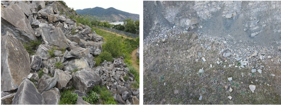
Fig. 27 Photographs of the deposition areas: left: Spitz with huge marble blocks versus right: Greifenstein with smaller sandstone blocks due to rather dense bedding
