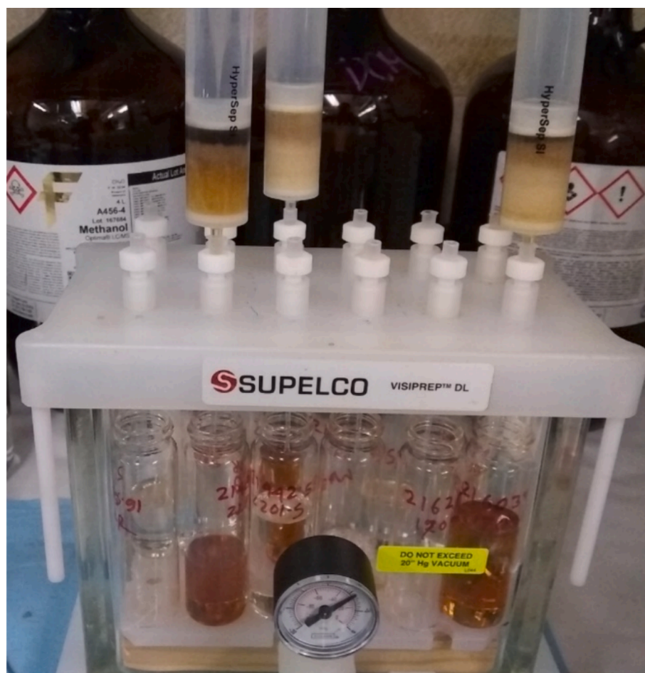
Fig. 2. The small-scale apparatus developed for SARA fractionation (reprinted from [49]).
