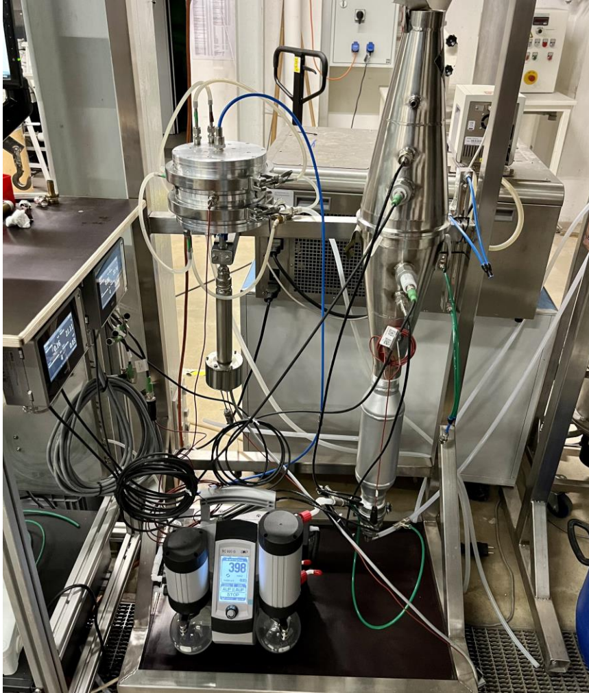
Figure 40: Experimental DAC plant set up in the Technikum at TU Wien. The system is shown in desorption mode. In the lower part of the picture, the vacuum pump can also be seen operating at 398 mbar.
