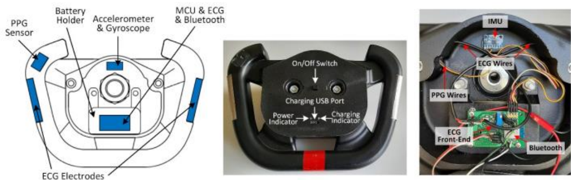
Figure 27: Smart steering wheel for unobtrusive health monitoring
