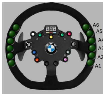
Figure 26: Smart steering wheel with sensors for hands on/off detection [29]
