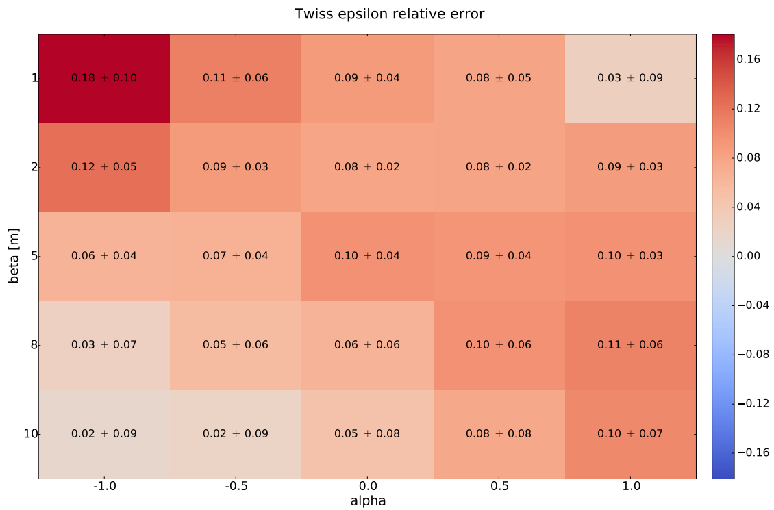
Figure 5.31: Relative error of the reconstructed Twiss \epsilon depending on the input beam distribution parameters, for bar of charge like distributions. The uncertainty shown is the result of the error propagation.
