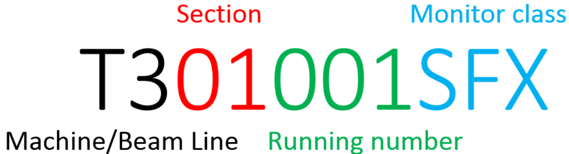
Figure 2.2: Example of the applied naming convention on a scintillating fiber hodoscope beam profile monitor in the transfer line to IR3.
