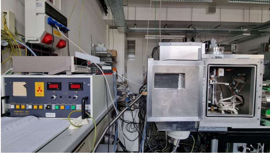
Figure 33: Photo of the complete spectrometer used for this work. From left to right, the setup is composed of the x-ray generator, the x-ray tube inside the shielding (behind the open chamber door) and the vacuum chamber.
