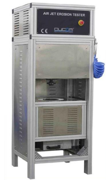
Figure 16 DUCOM Air Jet Erosion Tester
