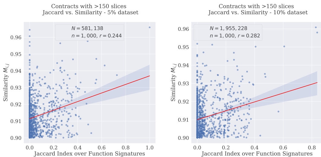
Figure 4.14: Correlation for the 10% and 5% datasets with limited number of slices. The red lines represent the line of best fit over the sampled observations. Compared to Figure 4.13, the correlation coefficient r is increasing when the matches are limited to those in which both contracts generate more than 150 slices.
