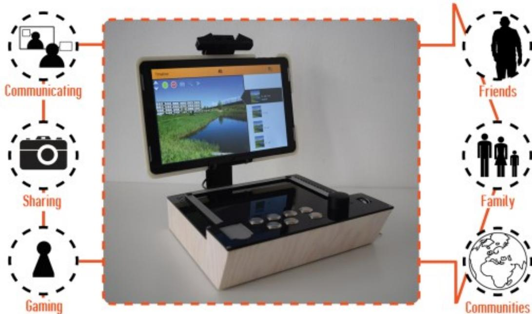
Figure 2.17: *KithNKin* prototype illustrating a standard tablet and a hardware platform for the tangible interaction [Con18a].
