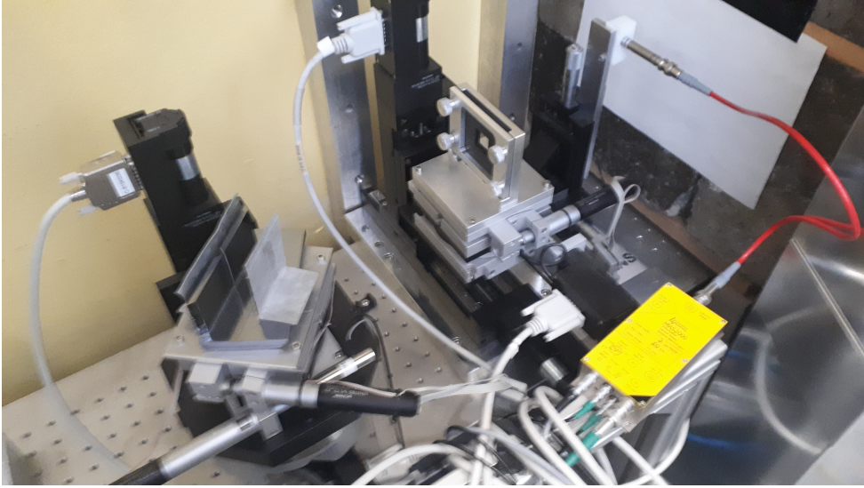
Figure 14: Installation of the incoming neutron monitor. The monitor is on the right side attached to a red cable. The sample holder with a screen is in the middle and on the left side the analyser can be seen.
