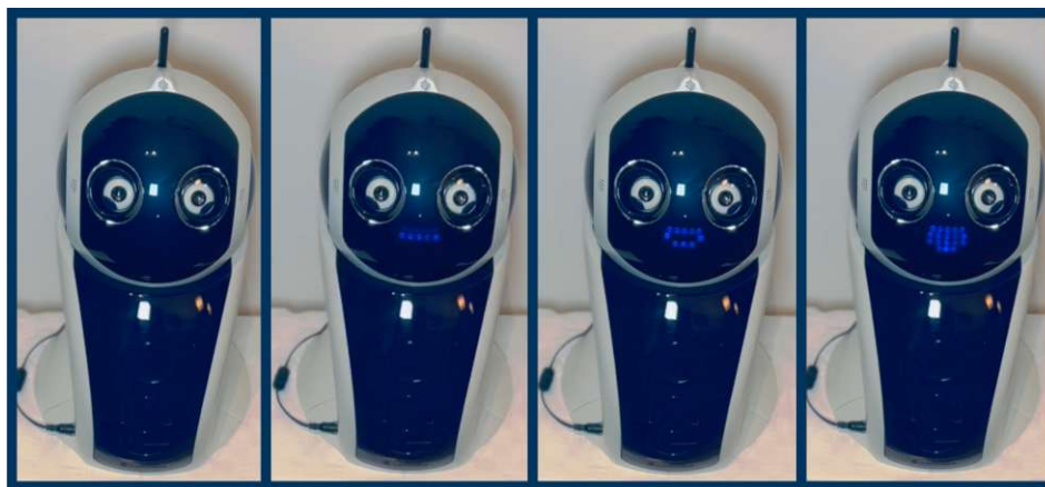
Figure 5.1: Subset of Q.bo One’s States – Vary in Number of Points the Mouth Consists of
