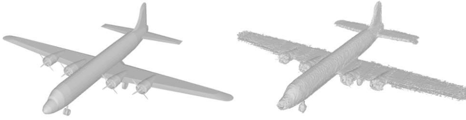
Figure 4.2: CAD Model (left) and TSDF reconstruction (right)
