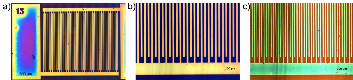
Figure S7: Micrographs of samples used for impedance measurements with interdigitating Pt finger electrodes beneath a \text{Ga}_2\text{O}_3 thin film. On one type of sample the electrode width and spacing are 15\ \mu\text{m} each – (a) and (b); on the second type of samples electrode width and spacing are 10\ \mu\text{m} each (c).
