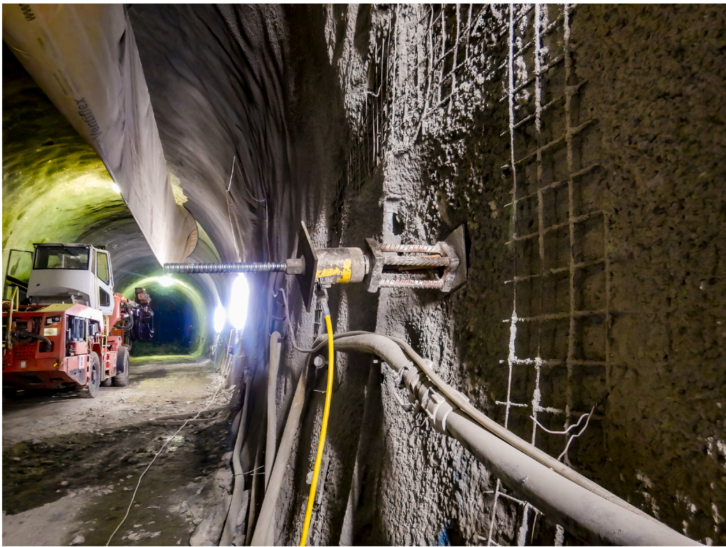
Fig. 2. Anchor pull test performed during the construction of ZaB research tunnel.
