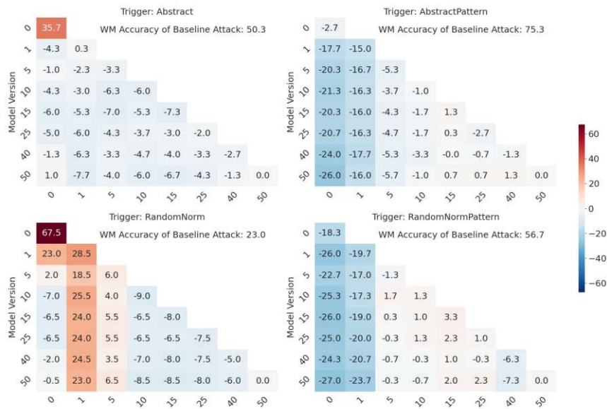
(a) Average difference in watermark accuracy to baseline attack. A positive value means the attack is less effective in removing the watermark than the baseline attack.
