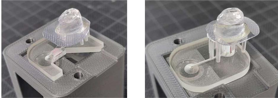
Figure 82: Combination of AuNP and blister device. Left: Variant I). Right: Variant II).
