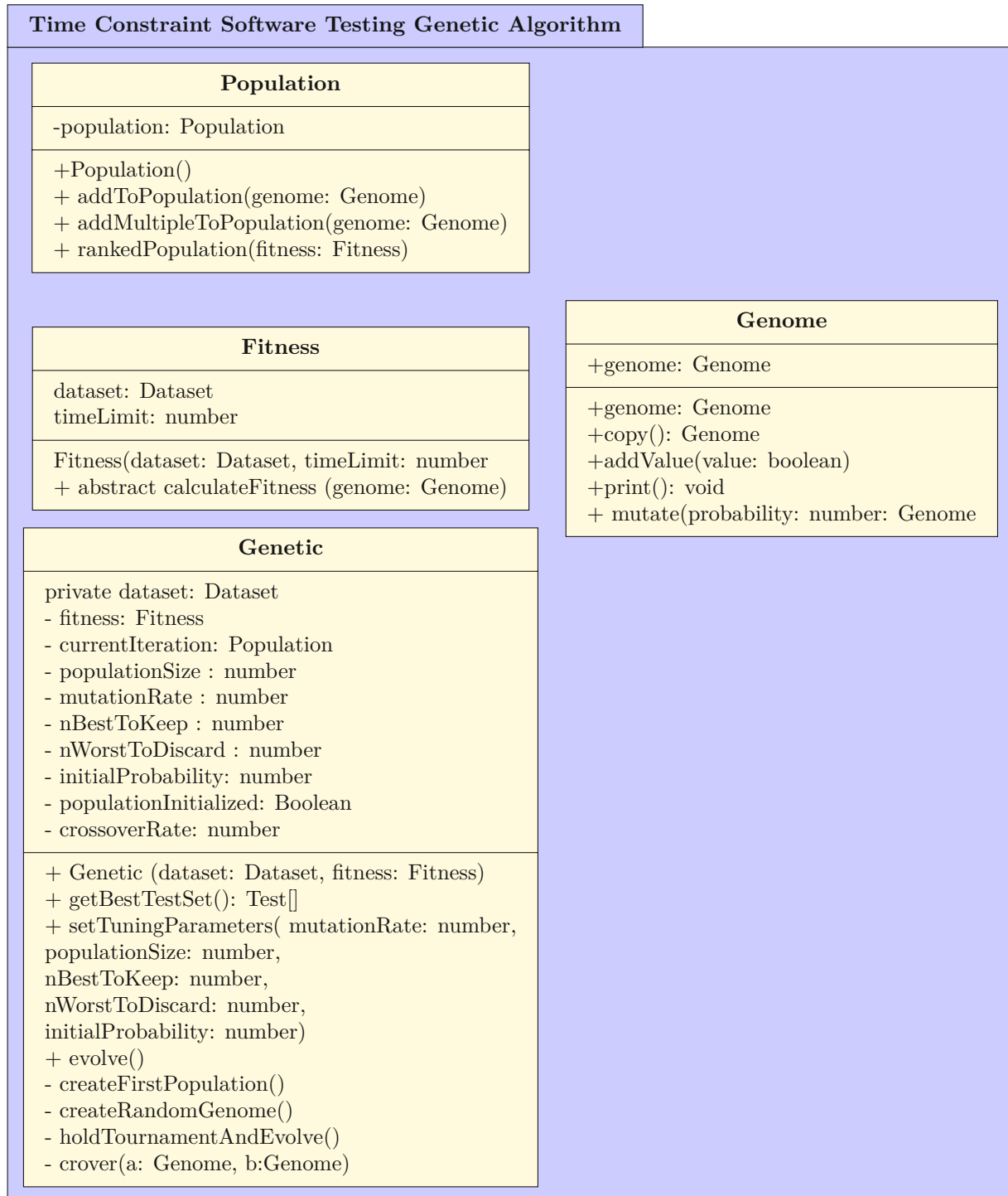
Figure 5.4: Iteration 2: Genetic algorithm architecture design
